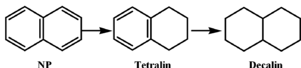
Fig. 4. Naphthalene hydrogenation reaction pathway.
